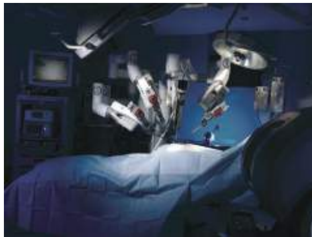
Figure 40-11. The da Vinci Surgical System used commonly for radical prostatectomy.
