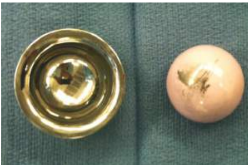
Figure 43-38. Failed ceramic on metal hip arthroplasty components. Note the metallic staining on the ceramic femoral head.
