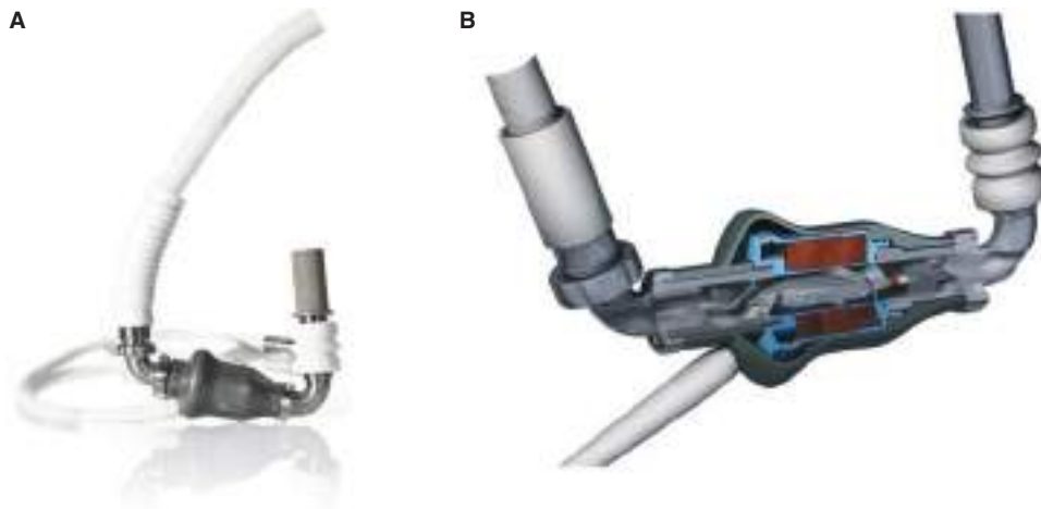
Figure 21-13. The HeartMate II LVAD viewed from the (A) outside and (B) inside. The device is an axial flow, rotary pump that produces no pulsatile action. The pump contains a magnet, and the rotor assembly functions by the electromotive force generated by the motor. The result is that blood is propelled from the inflow cannula to systemic circulation at flows up to 10 L/min. ( HeartMate, HeartMate II and St. Jude Medical are trademarks of St. Jude Medical, LLC or its related companies. Reproduced with permission of St. Jude Medical, ©2017. All rights reserved. )
